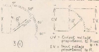
the potentiometers from external loading which would alter their resistance. These dc. amplifiers in turn are supplied from electronically regulated supplies and balanced to prevent spurious outputs. The potentiometer sliders, although they could be set manually, are driven by servo systems which could be operated from punched tape - even push buttons. The course computor would supply as its answer either a punched tape for feeding to the automatic pilot or a series of setings for same.
